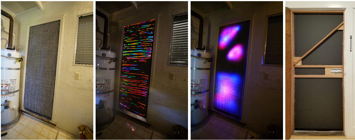
Figure 12: Leftmost: a wooden door. Next: results of rolling the RGB LED, microphone, transducer assembly back and forth across the door. Note that we can see the otherwise hidden heavy metal lock mechanism of the door, but we don't see so well the details of the fine structure. Next: results of a non-contact version of the new imaging modality which will be described in the next subsection. Here we can clearly see the various vibrational modes of the door, especially the lower portion which is very loose and rattles a lot. Rattling produces higher harmonics. The apparatus finds the natural resonant frequencies of each part of the door. The lower part of the door resonated around 55 CPS (Cycles Per Second). The left part resonated around 100 CPS, and the right part around 130 CPS. Rightmost: the true structure behind the door, showing the other side of the door (inside). Image is left-right reversed to match the other side of the door.
