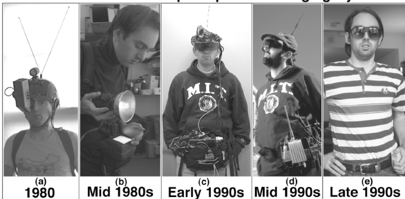
Figure 2: Evolution of the author's WearComp invention.
