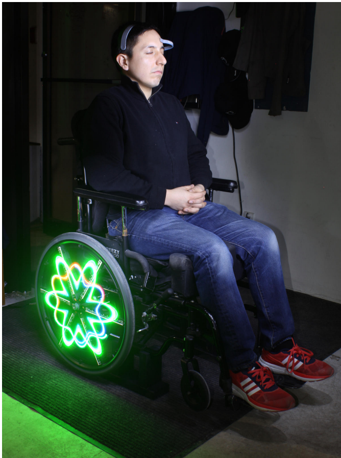
Fig. 11. Wheelchair sculpture shown here being controlled by brain-sensing headwear (Neurosky). Multiple players compete to calm the electrical signals fed to the motor, and provide purposeful rotary drive. On this wheel there are six SWIMs (Sequential Wave Imprinting Machines), which allow others to see the rotating magnetic field in the motor, and thus infer some aspects of the participant's brainwaves.
