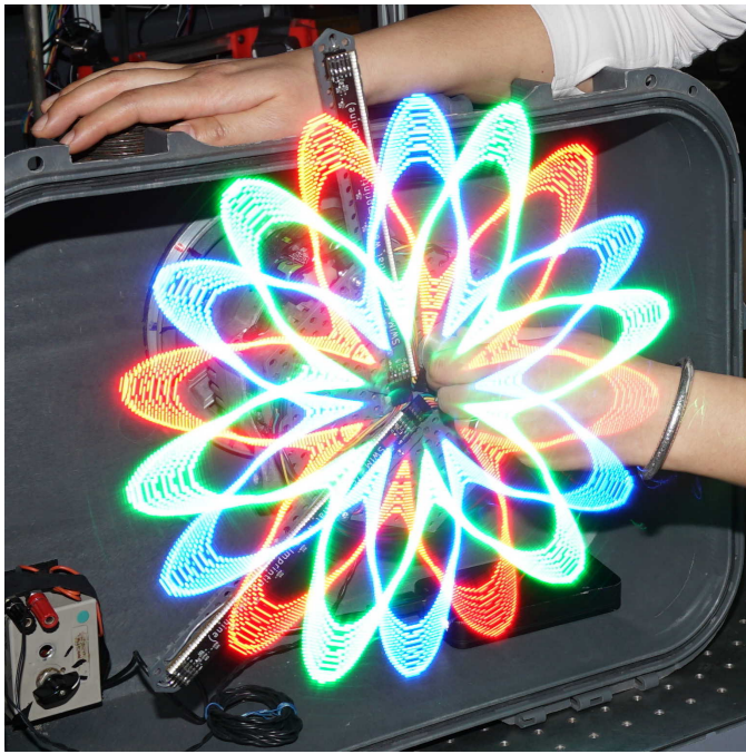
Fig. 9. The rotating magnetic field in a three phase motor is made visible with three rotating SWIMs. Here we see a variety of field strengths, as the field decays toward zero.
