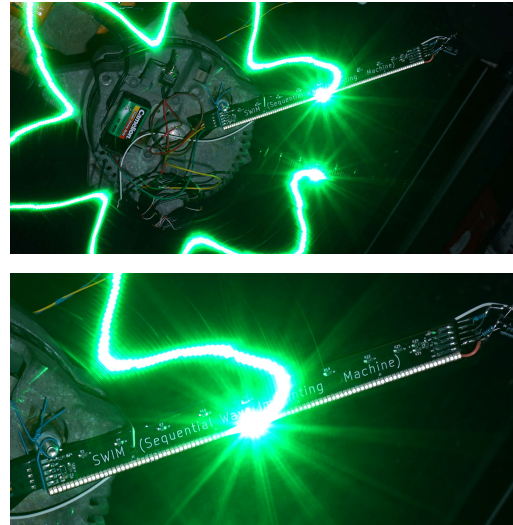
Fig. 8. A rotating SWIM allows us to see the rotating magnetic field in an electric motor. For the study of motors, we constructed a linear array of 100 LEDs to attach to the body of a motor. The array is connected to one of the motor's "stator" coils while the role of rotor and stator are reversed (i.e. the "stator" spins with the SWIM, while the "rotor" remains fixed in a vice on a workbench.
