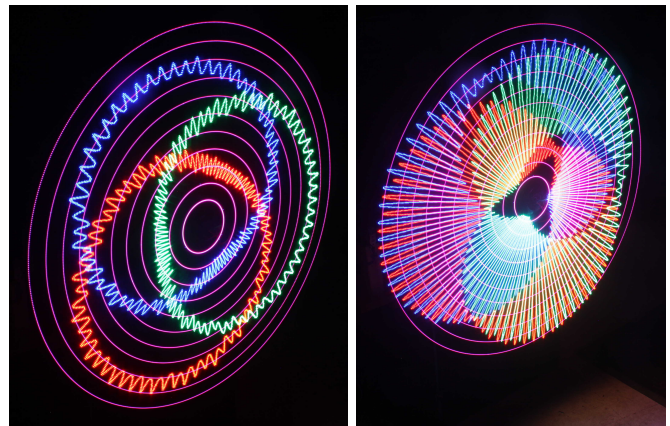
Fig. 10. Motor mindfulness. Top image: participant not in the state of flow, motor not turning. Next image: participant's brainwaves causing the motor to turn, while it also reveals its internal rotating magnetic field. Here we can see the field rotating around the 72 stator slots of this two-pole three-phase motor. Photograph taken with electronic flash. Typically, however, the experience takes place in a dark room with the lights off, as shown in the photographs on the bottom row, for various electric field currents and motor speeds as controlled by neurofeedback.
