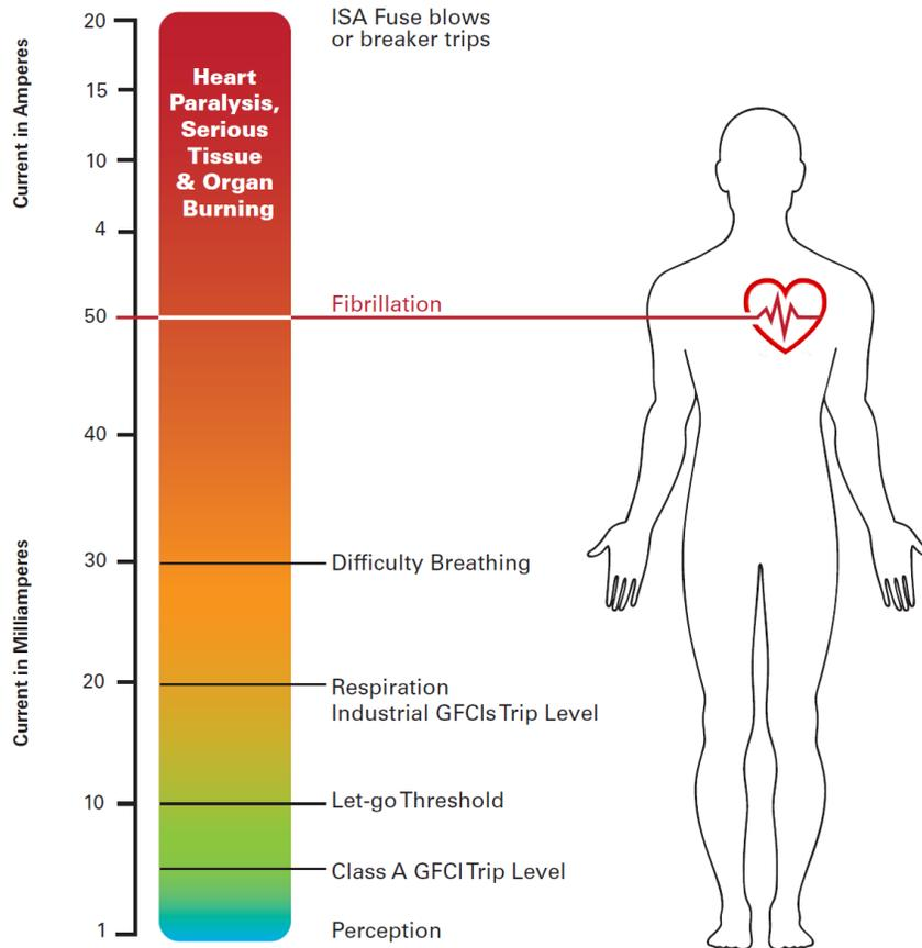
Figure 5. Current Flow Effect in Human Body
